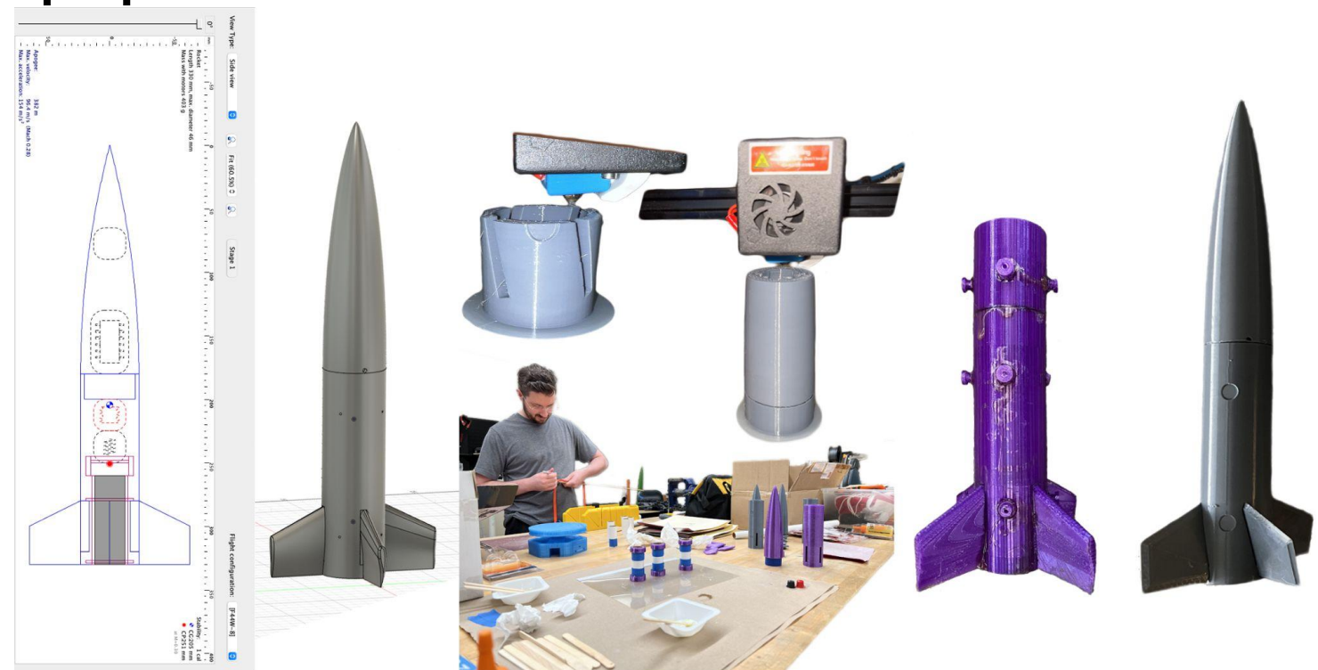
Left to right: OpenRocket file, Fusion file, 3D printing in progress, build in progress, completed rocket
