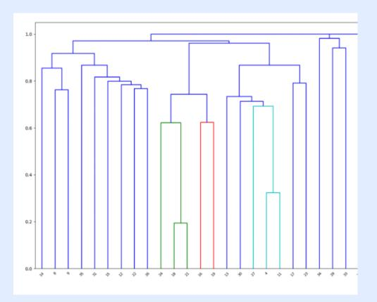
Lines are then compared based on the varying of "on" and "off" over time, and clustered together if deemed similar enough by set parameters.
