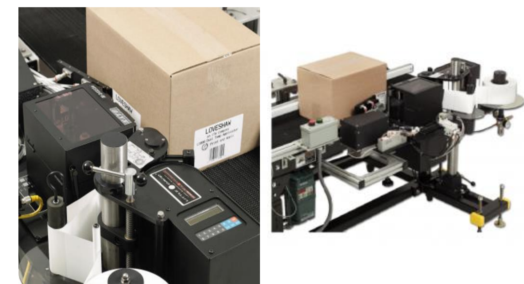
Automated print and label machine recommended to one facility, which improved productivity and limited energy.
